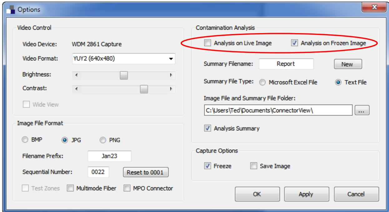
Choose whether to analyze a live image or analyze from the frozen image. If analyzing the frozen image the probe may be removed from the adapter or connector if you wish.
