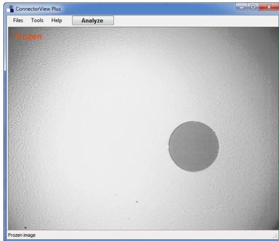
Here we are using the “Analysis on Frozen Image” setting. Analysis can also be do on the live image.
